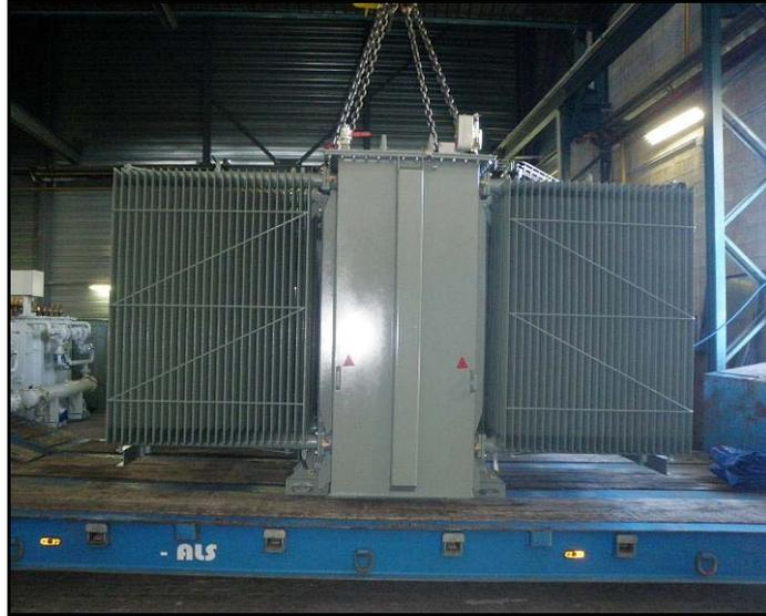
The unit must be on a wooden floor and rest on the substructures only. It must be carefully shored in both directions using wooden parts applied against the substructures. It must be securely slinged by lifting rings so as to seat it firmly on the floor and prevent it from tilting.
